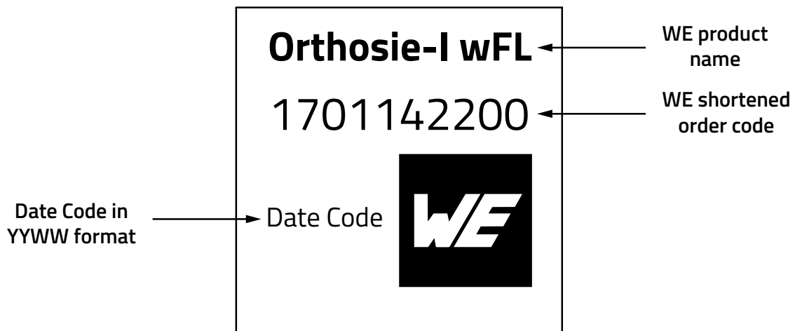
Figure 18: Label of the Orthosie-I with RF connector
